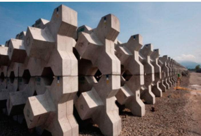
XBlocs storage and curing
