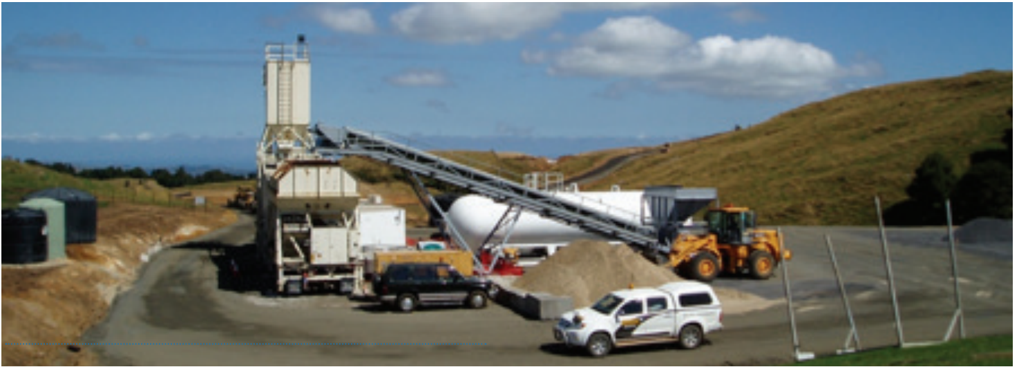
Example of a mobile concrete batching plant operation.
