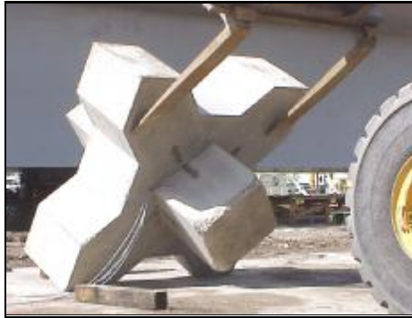
Figure 2: Photograph of Overturning – Cubical Leg test set-up.
