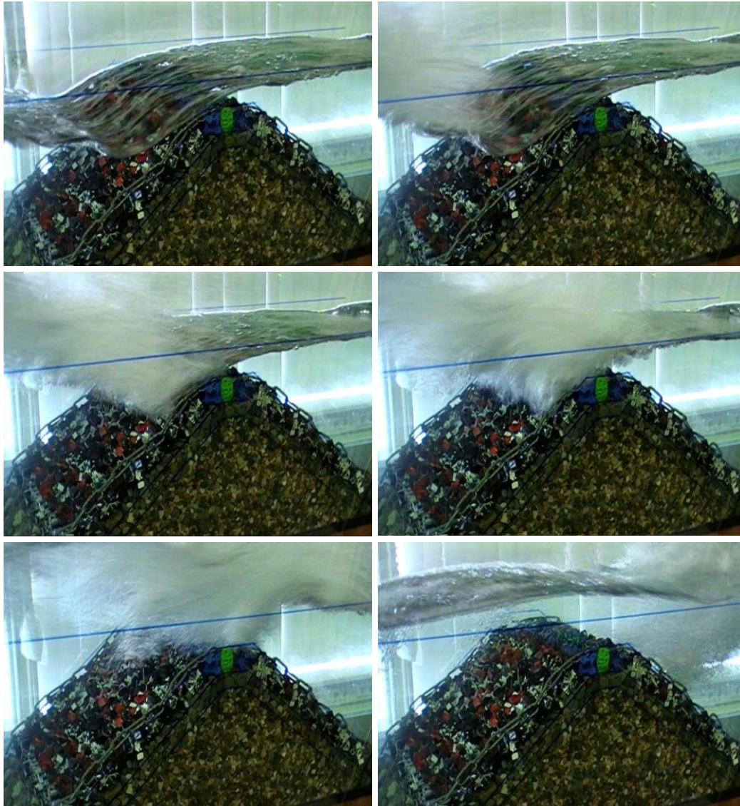
Figure 1: Wave passing over low crested breakwater with a narrow crest (van der Linde, 2010)
