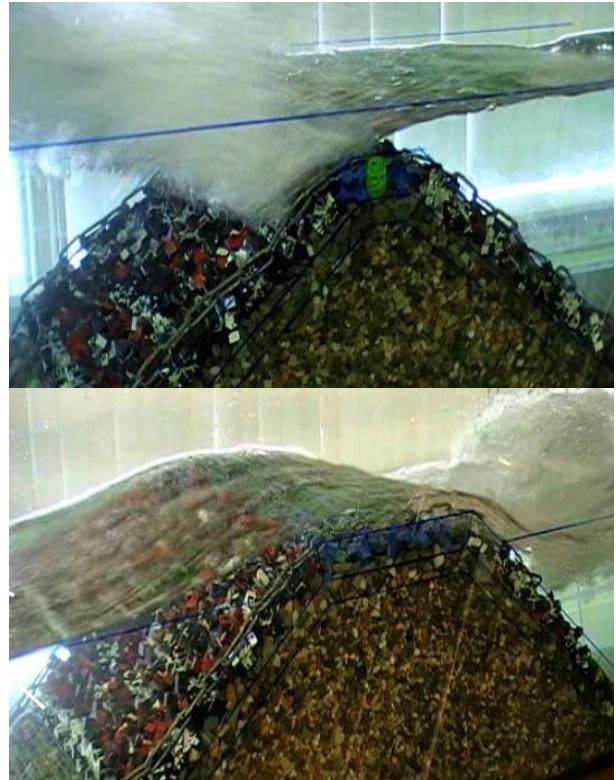
Fig. 1 Wave attack on submerged breakwater (with narrow crest, top) and low crested breakwater (emerged, with wide crest, bottom).
