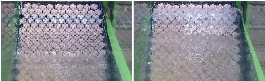
Figure 11. Still from video showing voids between the two rows of XP-Overtop (left) and overtopping wave travelling through (right)
